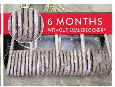
ScaleBlocker® is recommended for steamers to help minimize limescale buildup and corrosion, which can dramatically affect the operation of your equipment, resulting in downtime or service calls. It's a safe and economical way to maintain your investment.
